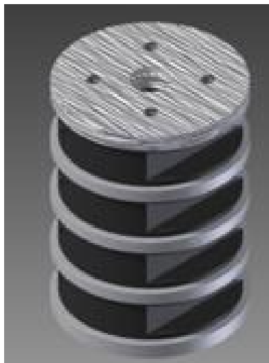
Figure 10. Computer model of the mechanical neckform used for all impact trials.
