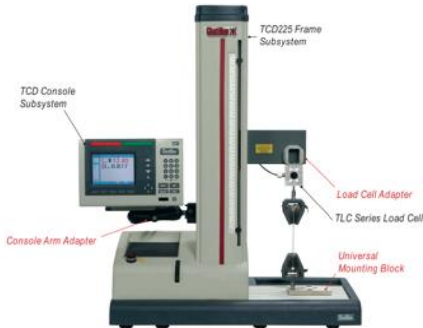
Figure 8. Chatillon® TCD1100 force tester by AMETEK Inc. Image of the force tester used in this study. Adapted from “Chatillon® TCD Series Console User’s Guide”, Ametek Industries, 2008, p. 1-2
