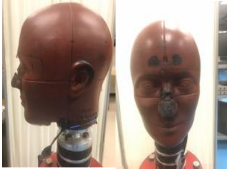
Figure 9. Photograph of the NOCSAE headform used in all impact trials.
