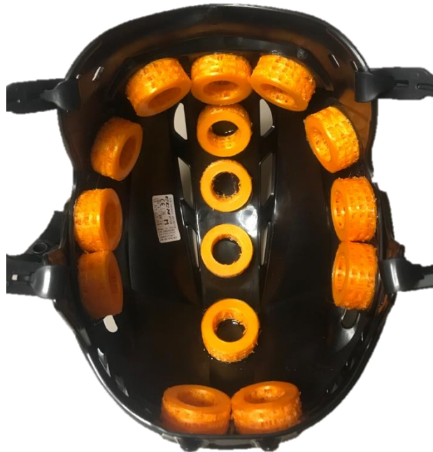
Figure 14. TPU lined helmet used for this study.
