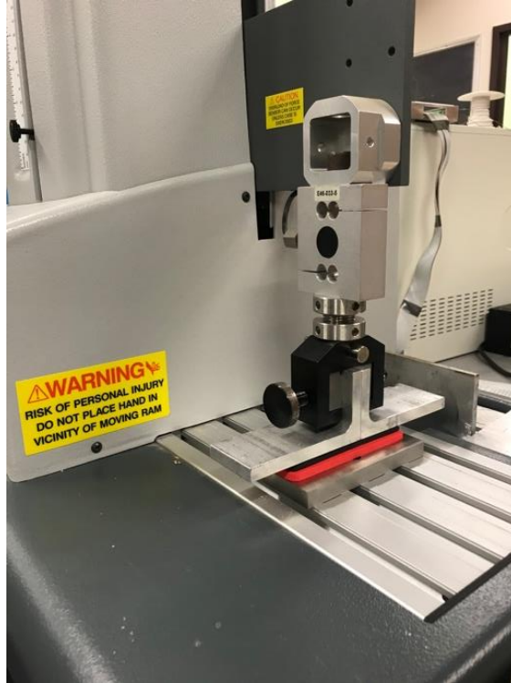
Figure 7. Set up used for static testing of the VN sample. Close up image of the VN sample during static testing with the Chatillon® TCD1100 force tester.
