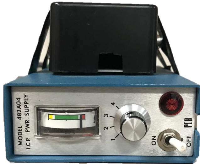
Figure 11. Power supply unit with amplifier for three channel signal processing.
