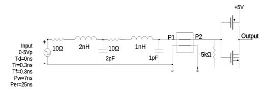
Figure 4.21: Transmission line circuit schematic.
