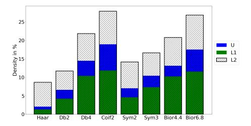
Figure 5.4: Average density of the  $L_1$ , U, and  $L_2$  matrices for the inverter chain circuit.
