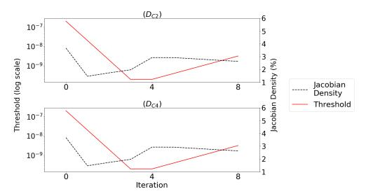
Figure 4.18: Variation of h and Jacobian density at each iteration for the ultrasound transducer driver using the Db4 wavelet.
