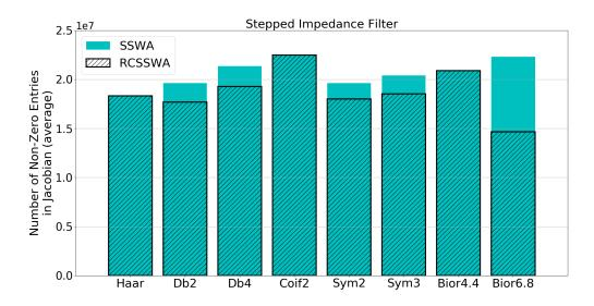
Figure 5.19: Average number of non-zero entries in the Jacobian matrices for the stepped impedance filter circuit.
