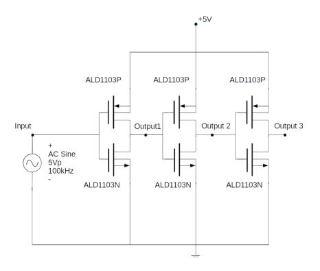
Figure 4.1: Inverter chain schematic.
