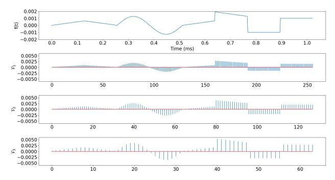
Figure 2.5: Scaling coefficients of a function, f(t), with the Haar wavelet at three scales. The resolution becomes coarser with each increase in scale. The wavelet transform for this example was performed with the discrete wavelet transform described in Section 2.3.4 with an f(t) discretized into 512 samples.
