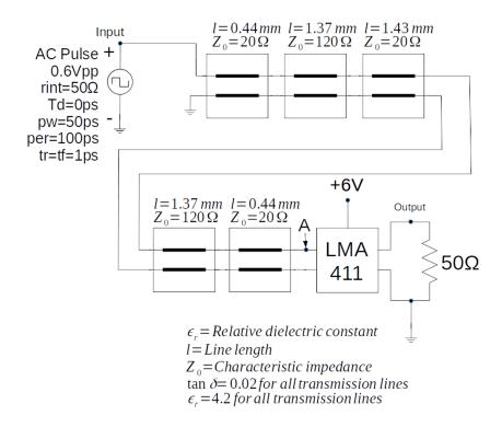
Figure 4.27: Stepped impedance filter circuit schematic.
