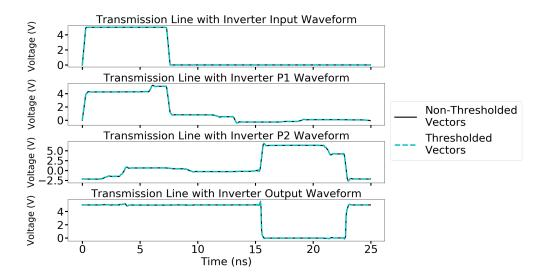
Figure 4.22: Input and output waveforms for the transmission line circuit. Dashed line represents the signals after they are thresholded.
