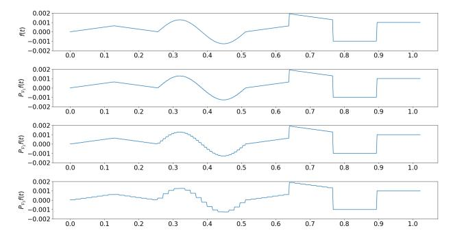
Figure 2.6: Approximation of a function, f(t), with the Haar wavelet at three scales. The resolution becomes coarser with each increase in scale. The wavelet transform for this example was performed with the discrete wavelet transform described in Section 2.3.4 with an f(t) discretized into 512 samples.
