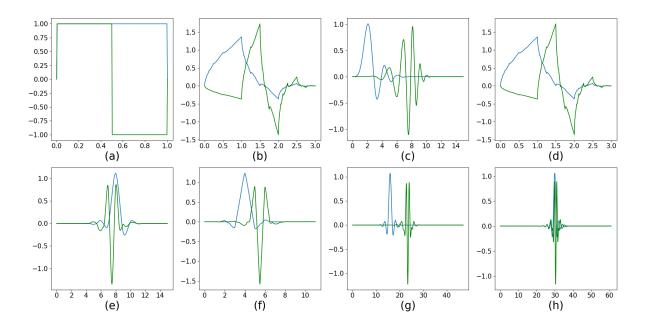
Figure 2.8: Commonly used orthogonal wavelets. Scaling function in blue and wavelet functions in green.
