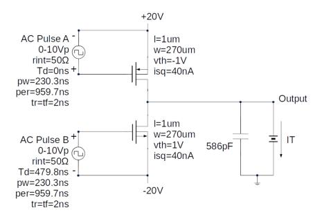
Figure 4.13: Ultrasound transducer driver schematic.
