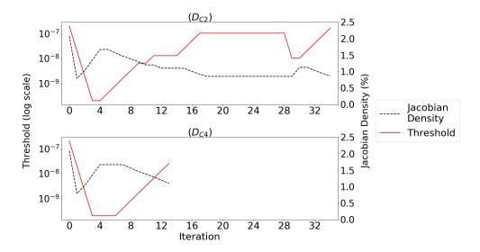
Figure 4.24: Variation of h and Jacobian density at each iteration for the transmission line circuit using the Haar wavelet.
