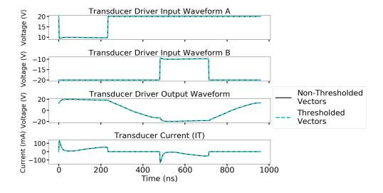
Figure 4.14: Input and output waveforms for the ultrasound transducer driver. Dashed line represents the signals after they are thresholded.
