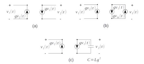
Figure 2.2: Gyrator and gyrator devices. (a) A simple gyrator, (b) an ideal voltage source, and (c) an inductor made from a gyrator and a capacitor. Note:  $v_{in}(t)$  is the voltage of the ideal voltage source.
