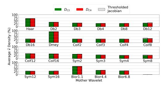
Figure 4.30: Average  $\hat{\boldsymbol{v}}$  densities for the stepped impedance filter circuit.
