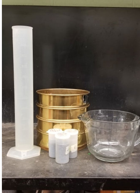
Fig 5.1: Geological sieves and graduated cylinder used for sieving soil samples. Soil was agitated in the measuring cup.
