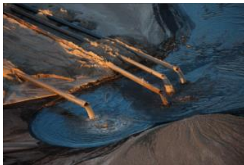
Figure 1.2: A series of oil-sand slurry pipes dispose slurries into tailing ponds. http://priceofoil.org/2014/02/24/tar-sands-tailing-ponds-leaking/
