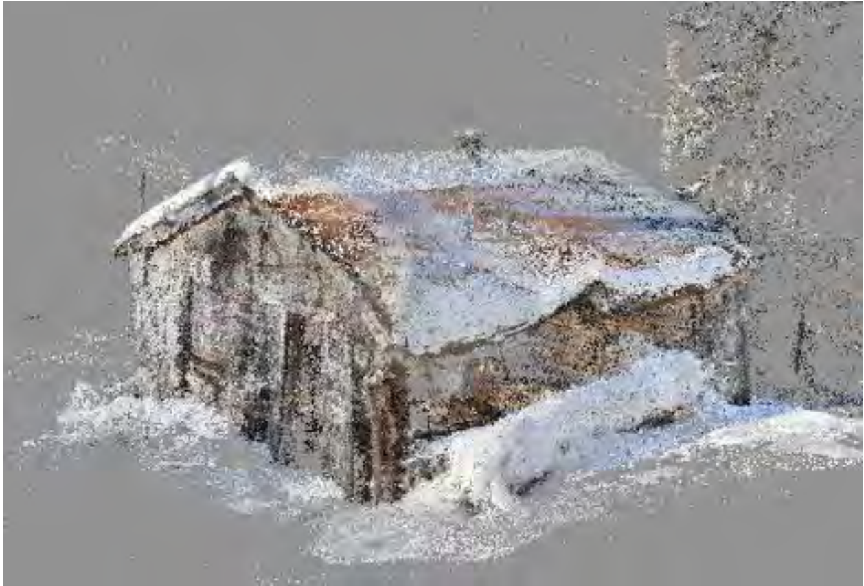
Plate E.15, Cabin 3, 3D model based on cloud points, utilizing DSLR photographs.
