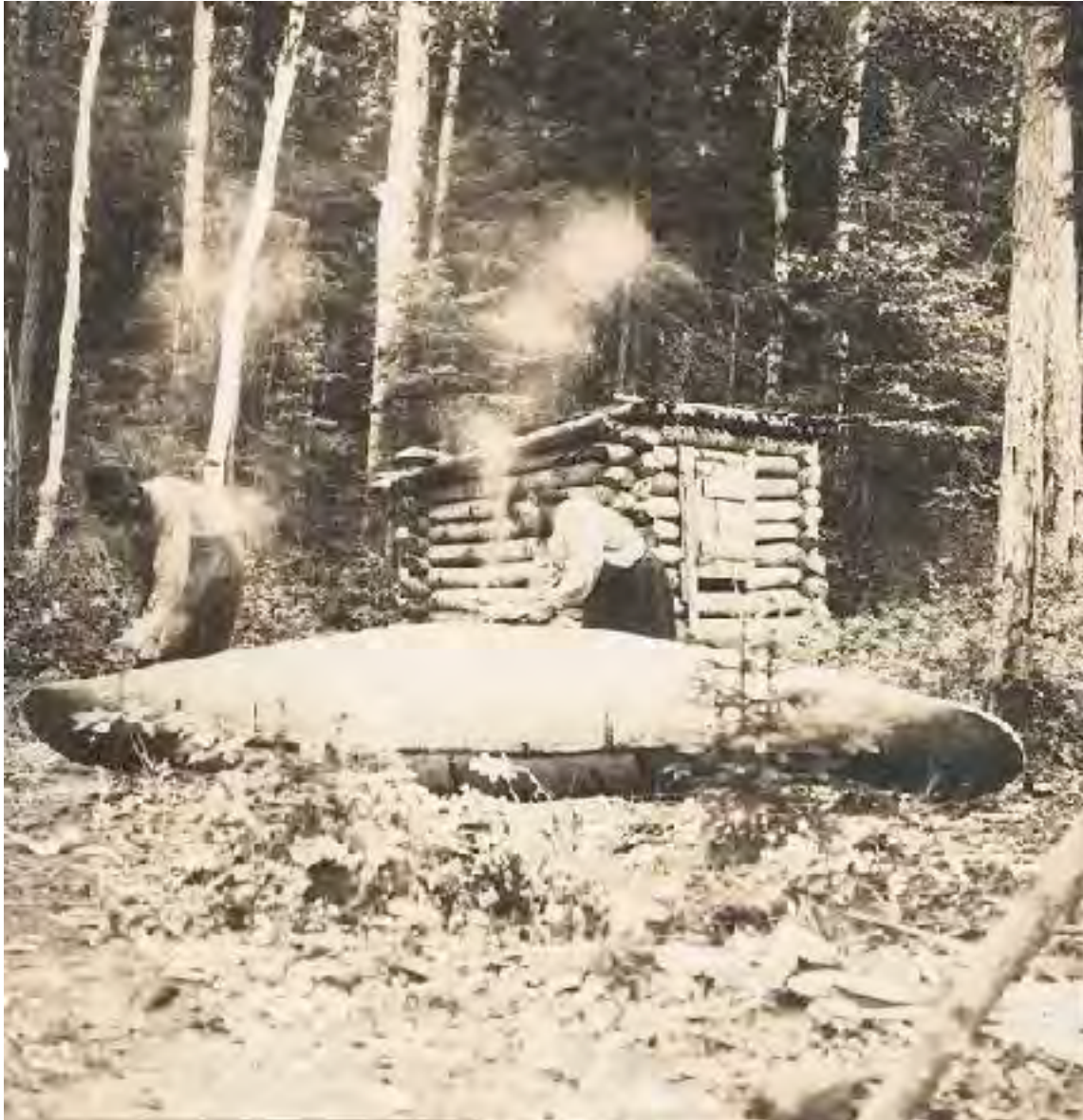
Plate B.10, Anishinaabeg man and woman applying pine or spruce pitch while building canoe, pantry or cold storage visible in background. Lac Seul First Nation, Taken by F.W. Waugh, 1919. Library and Archives Canada, Archives, Item number 5318567, http://central.bac-lac.gc.ca/.redirect?app=fonandcol&id=5318565&lang=eng
