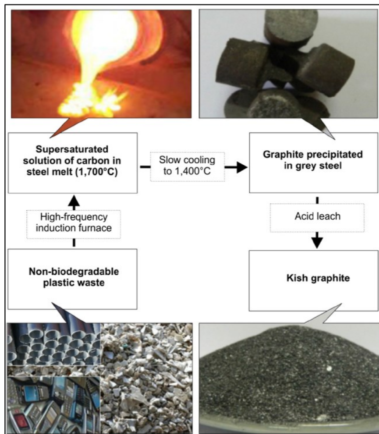
Figure 1.3 Procedure for preparation of kish graphite from plastic waste. Adapted from ref [12].
