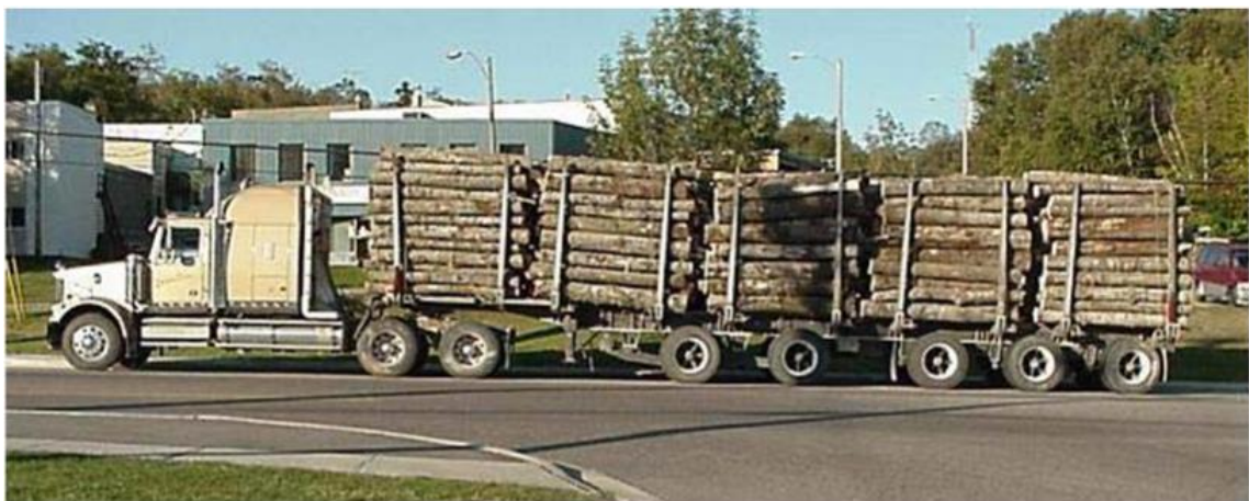
Figure 1. Typical log truck configuration in Ontario. Source: Hajek et al. (2008).
