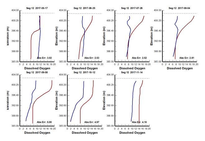
Figure 5.6.5. Dissolved oxygen calibration profiles with  $O_2$  calculations, SOD enabled. Field measurements in blue, model output in red. Total AME = 3.572 mg/L DO.
