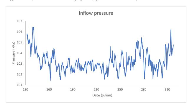
Figure 5.4.1. Barometric pressure sensor readings obtained from the HOBO data logger deployed in the inflow to Cleaver Lake.
