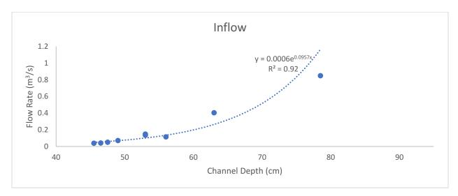
Figure B.3. Measured inflow rates plotted vs. channel depth and established regression equation used in correlating flows from pressure logging HOBO device for Cleaver Lake inflow.
