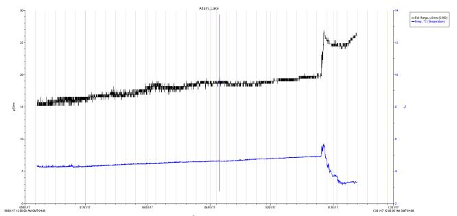
Figure B.2. Conductivity readings in  $\mu S/cm^2$  from HOBO device deployed at the bottom of Cleaver Lake from June 7 to November 13, 2017.
