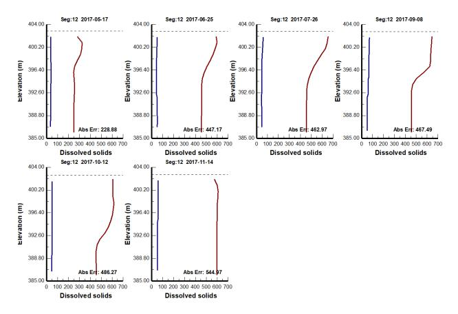
Figure 5.7.2. TDS calibration profiles for Cleaver Lake obtained during the operational experimental scenario utilizing modified inflow water quality characteristics. Modelled output in red, original field data in blue.
