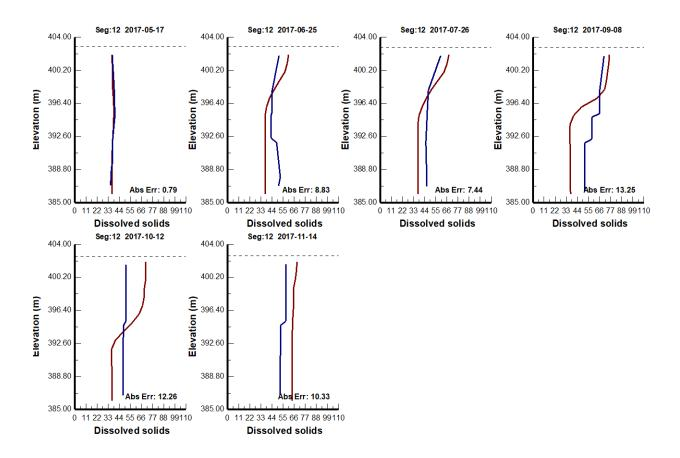
Figure 5.6.4. TDS calibration profiles for Cleaver Lake following temperature calibration and activation of water quality calculations. Total AME = 8.818 mg/L TDS.
