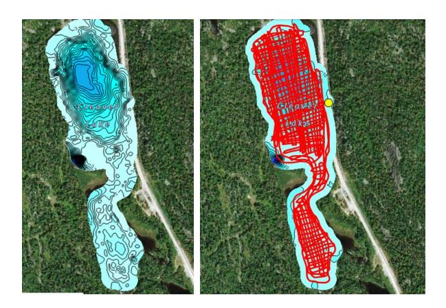
Figure 4.2.2. Bathymetric map (left) and GPS track (right) showing depth sounder collection route for Cleaver Lake.
