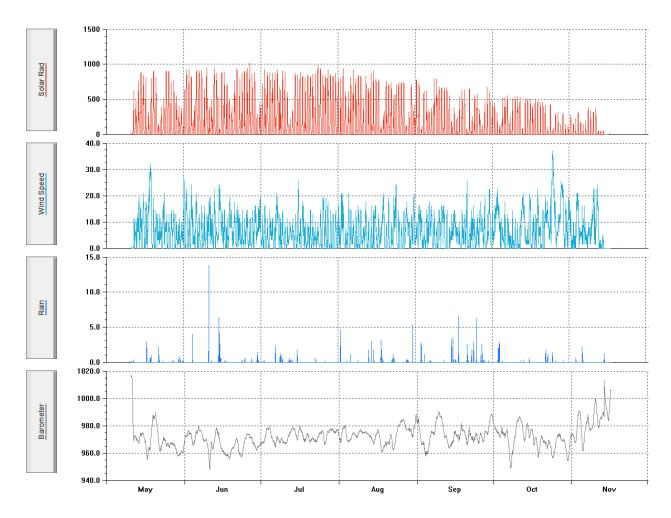
Figure 5.4.3. Boundary condition data obtained from the Davis instruments weather station deployed at Cleaver Lake for the modelled time period. Moving from top to bottom, the uppermost chart depicts solar radiation in W/m², the next displays wind speed in km/h, the third shows recorded rainfall in mm, and the bottom chart depicts barometric air pressure in mbar.
