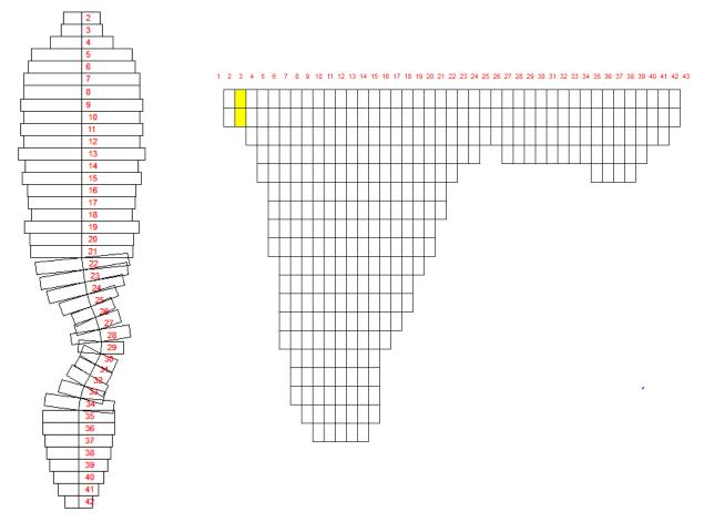
Figure 4.2.1. Top view (left) and side view (right) of the CE-QUAL-W2 computational grid for Cleaver Lake.
