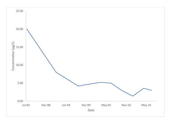
Figure 5.1.3. Total copper concentrations in  $\mu$ g/L for the inflow to Cleaver Lake from October 1983 to September 2015. CWQG limit for total copper = 2  $\mu$ g/L, zero-effect concentration for Brook Trout = 3-5  $\mu$ g/L (Sauter, 1976).
