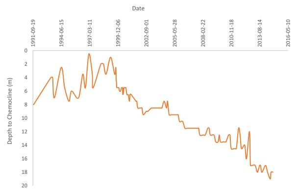
Figure 5.1.1. Depth to the chemocline (m) for Cleaver Lake from September 1991 to September 2015.
