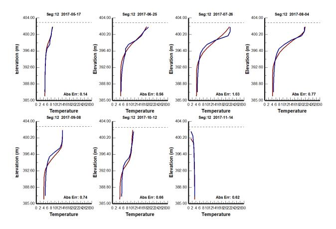
Figure 5.6.3. Temperature profiles for Cleaver Lake after final calibration adjustments with water quality calculations enabled. Field measurements shown in blue, model outputs shown in red. Total AME = 0.647°C.
