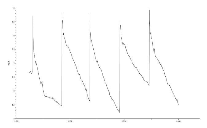
Figure 5.5.1. Dissolved oxygen values from a HOBO data logger used in the SOD chamber test. Five sediment core samples were tested on consecutive days at 20°C in a dark chamber, allowing 24 hours for oxygen consumption in each sample.
