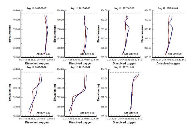
Figure 5.6.6. Dissolved oxygen calibration profiles for Cleaver Lake following addition of representative algal species. Field measurements in blue, model output in red. Total AME = 0.570 mg/L DO.
