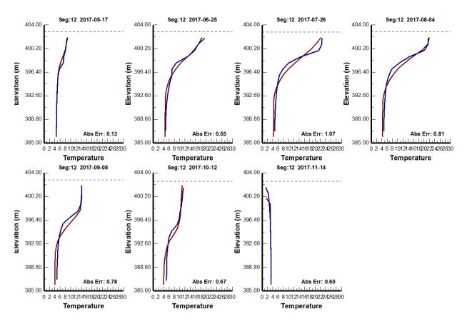
Figure 5.6.2. Temperature calibration profiles following inclusion of cloud cover, wind sheltering coefficients and adjustment of sediment temperature. Field measurements in blue, model output in red. Total AME = 0.657°C.
