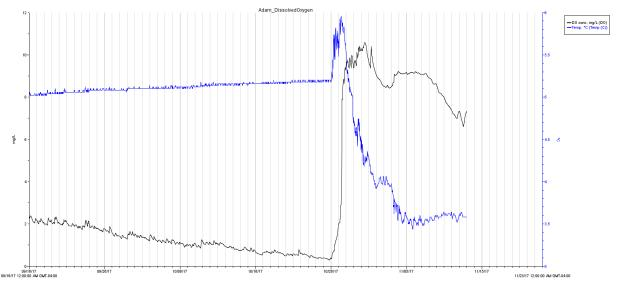
Figure B.1. Dissolved Oxygen and temperature readings from September 16 to November 13, 2017 obtained by HOBO dissolved oxygen probe.
