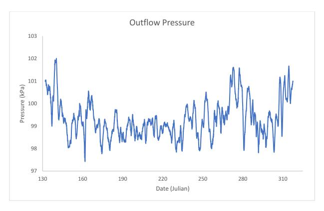
Figure 5.4.2. Barometric pressure sensor readings from the HOBO data logger deployed in the outflow from Cleaver Lake.
