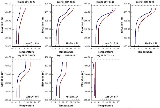
Figure 5.7.5. Temperature calibration profiles for Cleaver Lake in an experimental climate change scenario of +6.3°C annual average air temperature. Modelled output in red, field observed data in blue.
