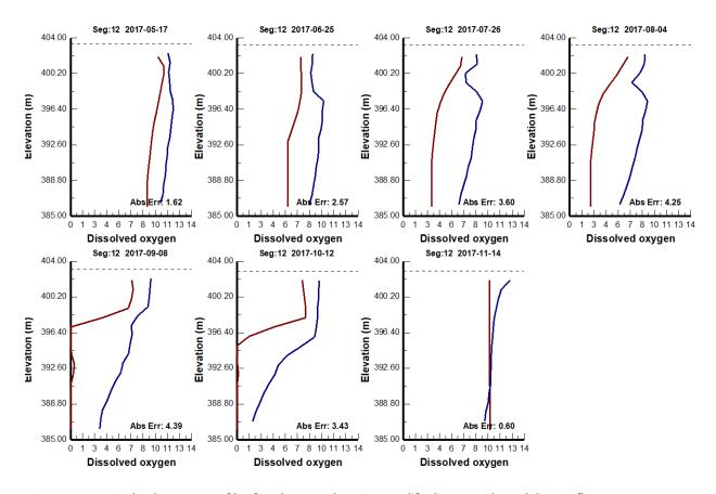
Figure 5.7.8. Dissolved oxygen profiles for Cleaver Lake using modified meteorological data, inflow temperatures and sediment temperature to represent a theoretical climate change scenario of +6.3°C annual air temperature. 2017 field observed values in blue, model outputs in red.
