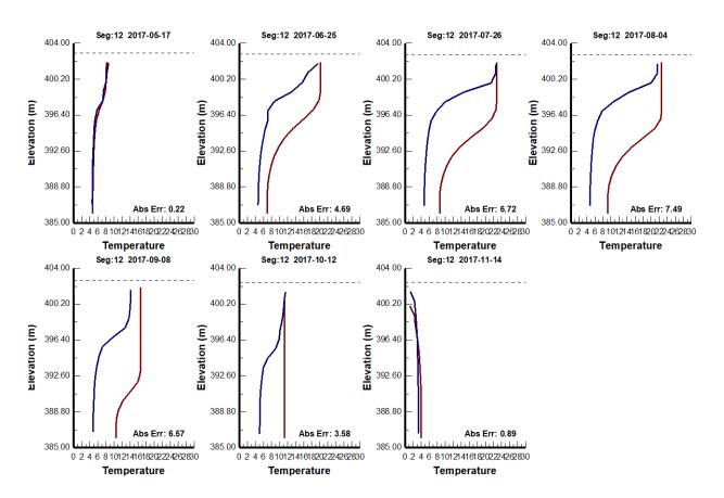
Figure 5.6.1. Temperature calibration profiles with unadjusted model coefficients, prior to cloud cover estimation and sediment temperature adjustment; wind sheltering, and water quality calculations disabled. Field measurements in blue, model output in red. Total AME = 4.31°C.
