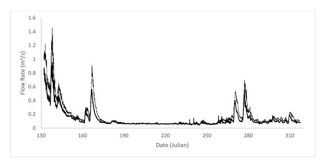
Figure 5.4.4. Calculated flow rates in m<sup>3</sup>/s used for CE-QUAL-W2 model input. Inflow rates represented by the solid line; outflow rates represented by the dotted line.
