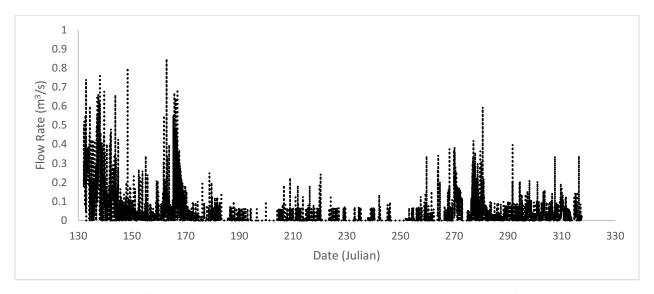
Figure 5.4.5. Additional flow rates to correct water balance within the CE-QUAL-W2 model of Cleaver Lake as calculated by the water balance utility. Rates were measured in m<sup>3</sup>/s.
