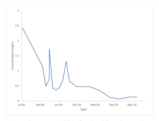
Figure 5.1.4. Total zinc concentrations in mg/L for the inflow to Cleaver Lake from October 1983 to October 2017. PWQO recommended value for zinc = 0.02 mg/L, zero-effect concentration for Brook Trout = 0.534 mg/L (Holcombe et al., 1979).
