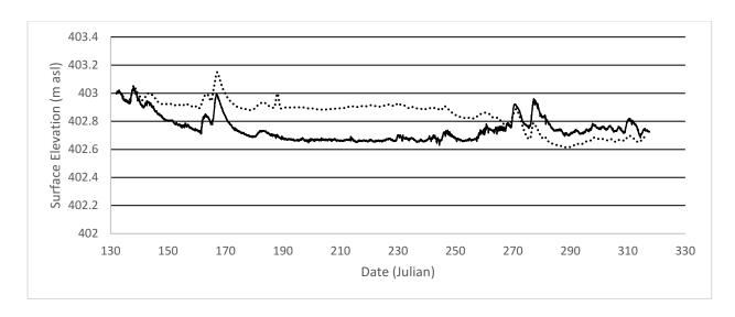
Figure 5.2.2. Water surface elevations for Cleaver Lake in metres above sea level as calculated from field deployed pressure sensor (solid line) and from model output (dotted line).
