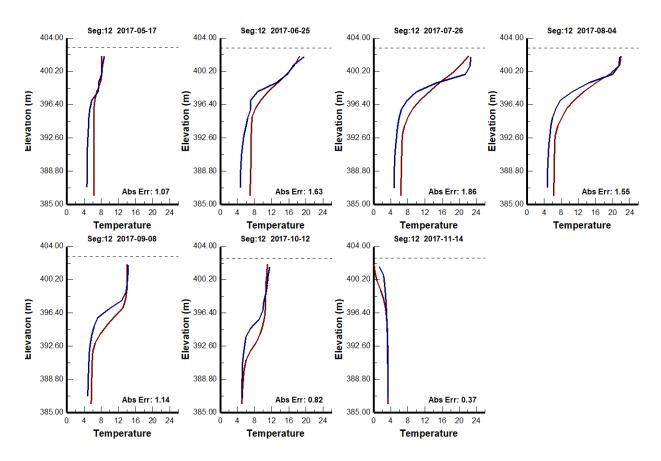
Figure 5.7.1. Temperature calibration profiles for Cleaver Lake in the operational experimental scenario using modified inflow water quality characteristics. Modelled output in red, field observed data in blue.
