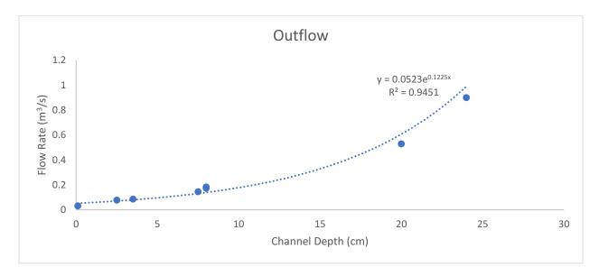
Figure B.4. Measured flow rates plotted vs. channel depth and the established regression equation used in correlating flows from pressure logging HOBO device for Cleaver Lake outflow.
