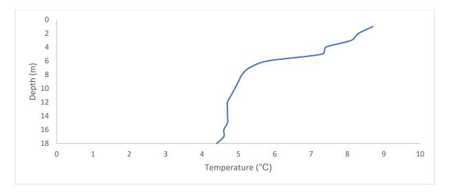
Figure 5.3.1. Temperature profile of Cleaver Lake from May 16, 2017 obtained in the deep profundal zone of the lake.
