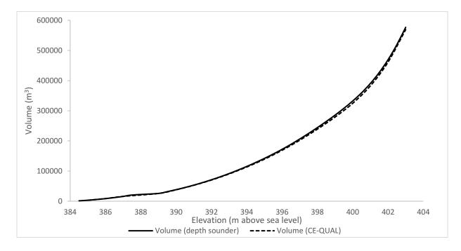
Figure 5.2.1. Volume-elevation graph for Cleaver Lake comparing field data from depth sounder with constructed CE-QUAL-W2 bathymetry grid data.
