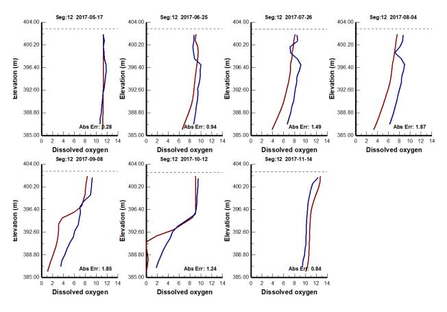
Figure 5.7.3. Dissolved Oxygen calibration profiles for Cleaver Lake in the operational experimental scenario with modified inflow water quality characteristics. Modelled output in red, field observed data in blue.
