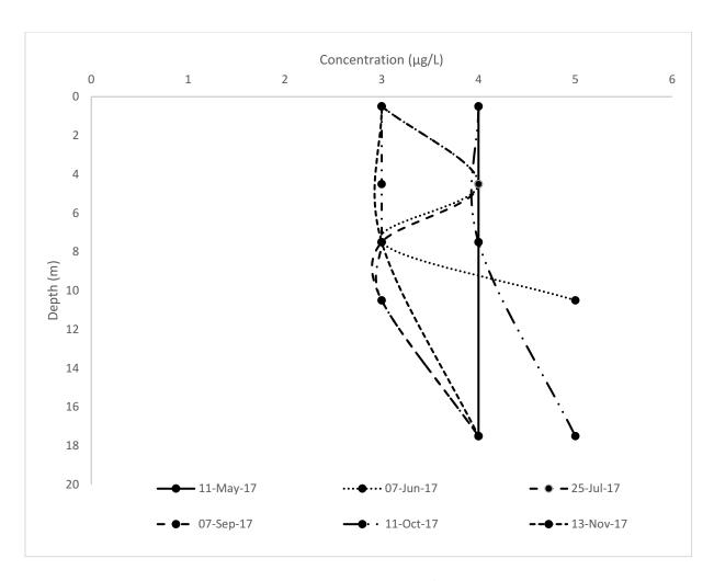
Figure 5.1.6. Total copper concentrations for 2017 field season in  $\mu g/L$  for Cleaver Lake profundal zone plotted vs. depth in metres. MDL = 2  $\mu g/L$ . Data points included.
