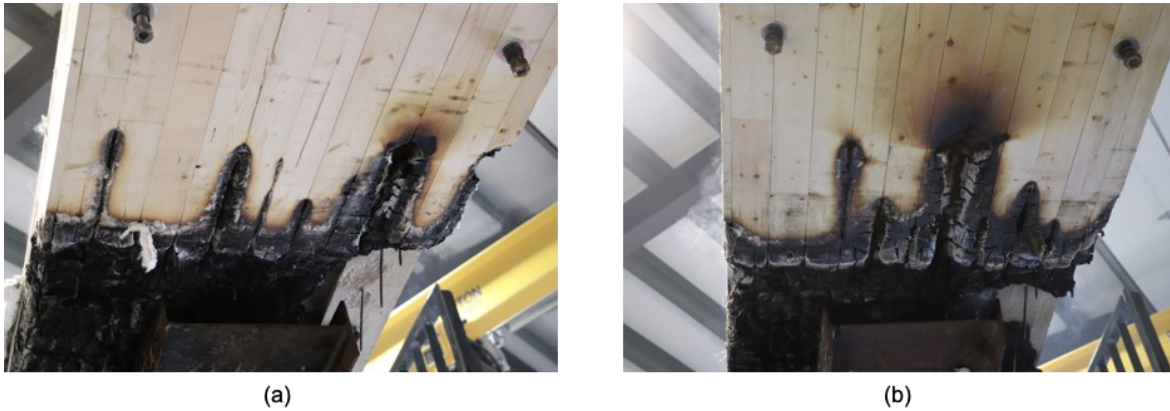
Figure 4.46: Fire spread and horizontal charring through the glue lines of the bottom ply.
