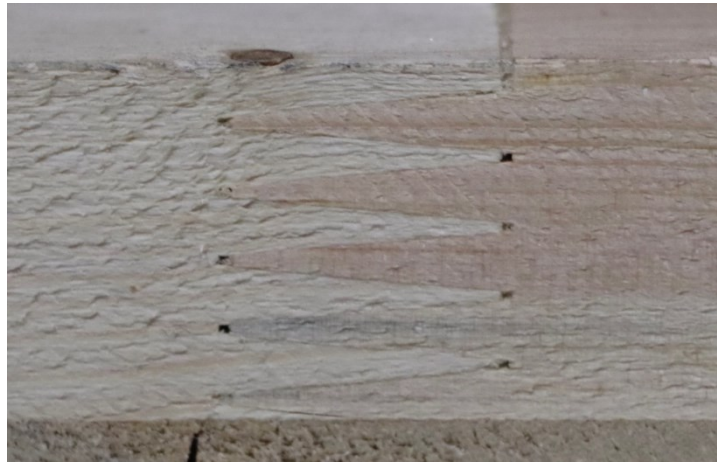
Figure 2.2: Typical CLT finger joint.
