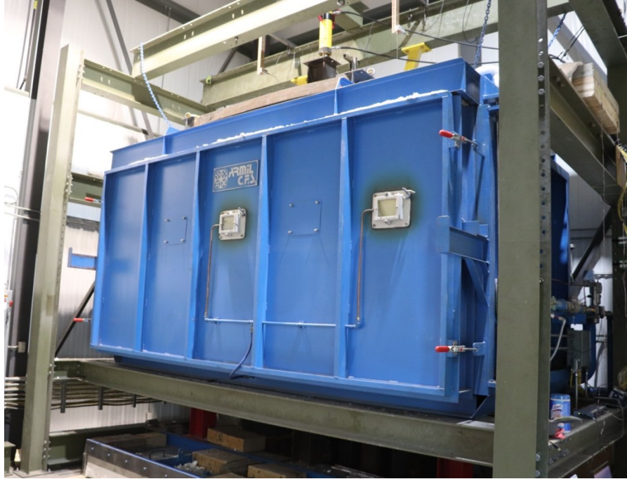
Figure 3.2: Large fire testing furnace accommodated at LUFTRL (Courtesy of Dr. Salem).
