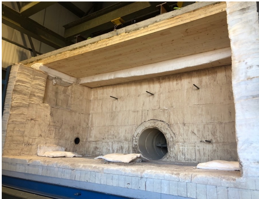
Figure 3.3: Interior of the testing furnace with one of the TCC floor test assemblies installed.
