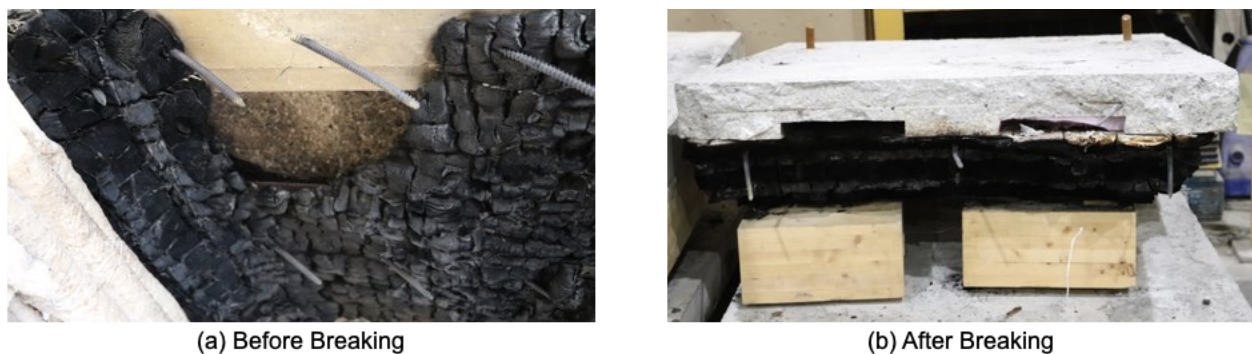
Figure 4.47: Loss of the insulation layer due to severe charring near the furnace wall.
