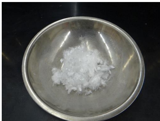
Figure 3.3. Polypropylene microfiber utilized in the FR-CPB preparation.
