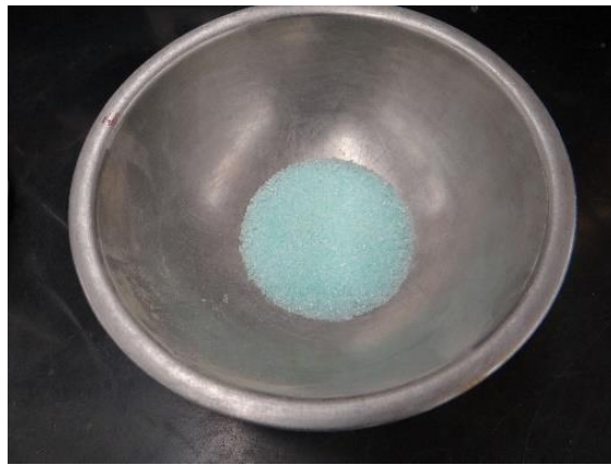
Figure 3.2. Sulfate salt utilized to create the required concentrations of sulfate mixing water.
