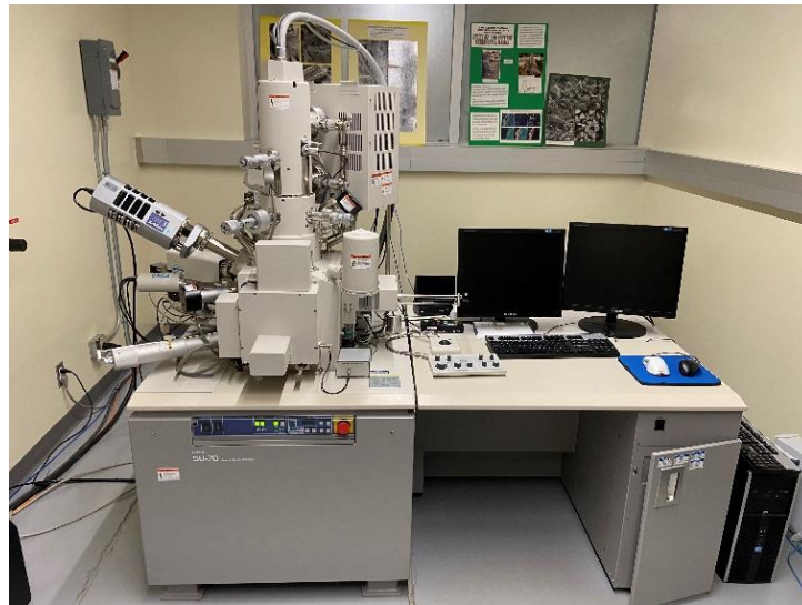
Figure 3.6. Scanning electron microscope used to capture the microscale SEM images of CPB and FR-CPB.
