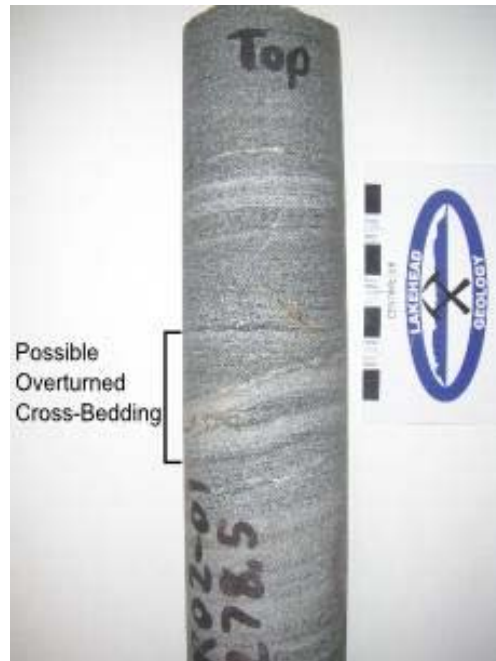
Figure 4.12: Core sample (Drill hole WR02-01, 278.5m) of metawacke with possible overturned cross bedding.
