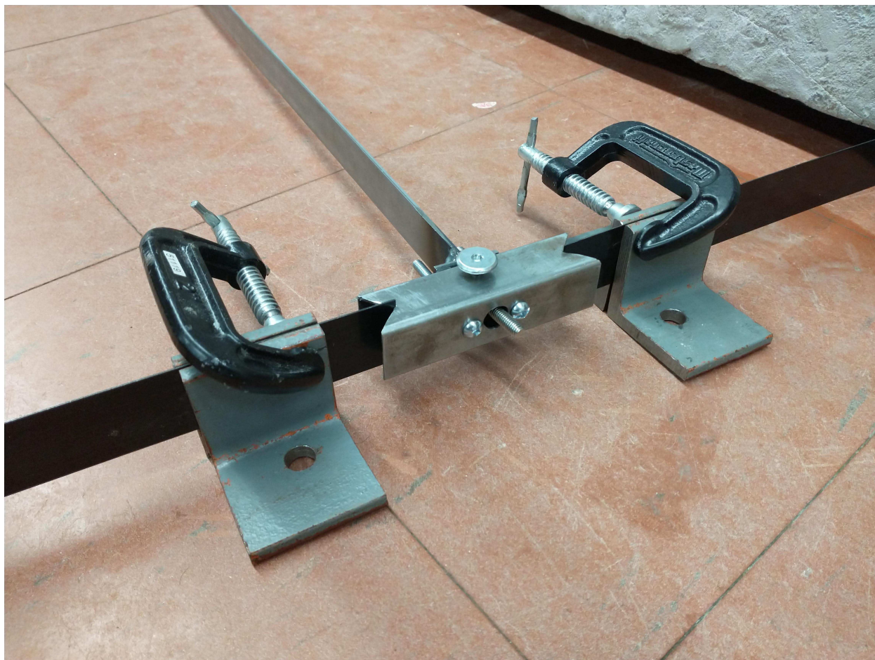
Figure 5.8: Photograph of the constructed connection (not attached)
