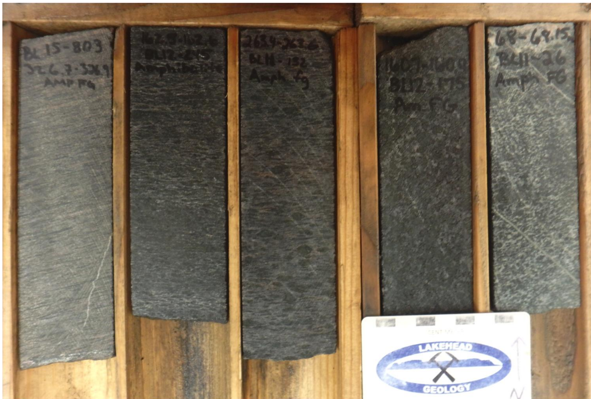
Figure 4.20. Core samples of amphibole felsic gneiss. The two core samples on the right display a massive texture with porphyroblastic amphibole grains within a felsic groundmass. Core samples in the center and to the left display an increasing foliation defined by amphibole and biotite porphyroblast tails.
