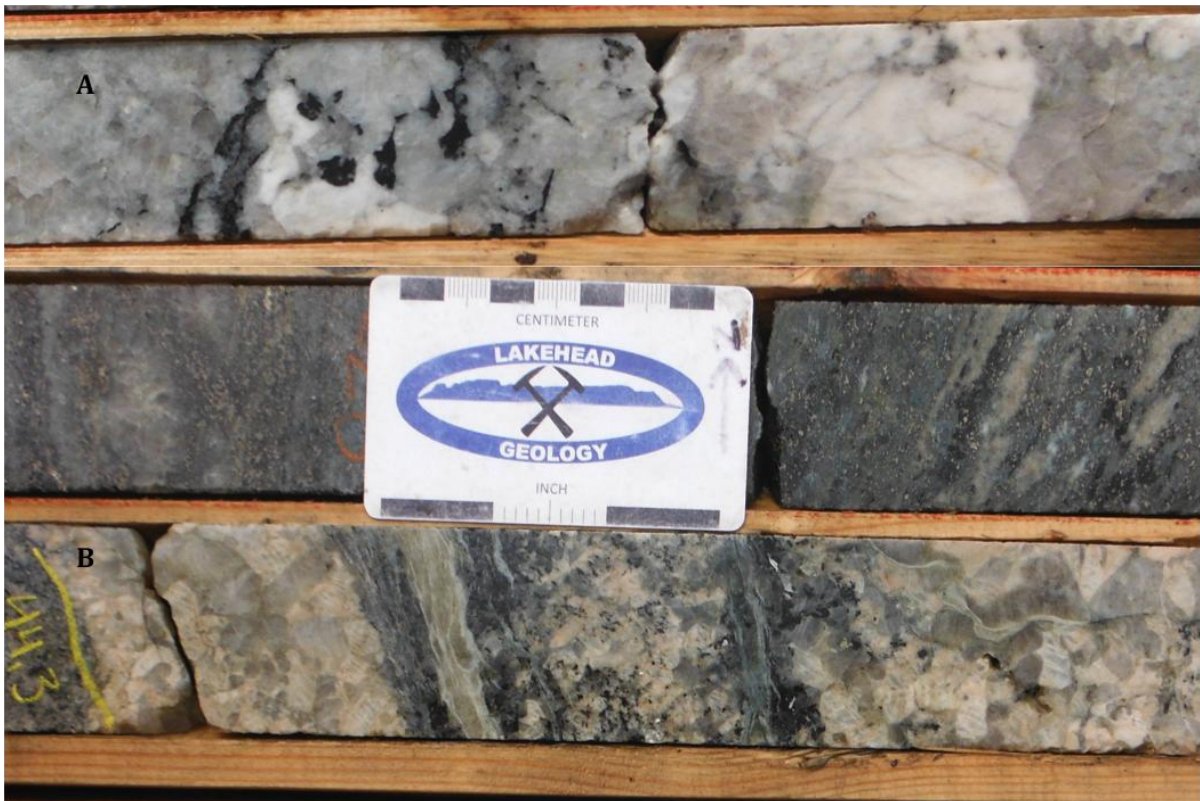
Figure 4.25. A) Coarse-grained, undeformed pegmatite. B) Strongly deformed pegmatite with increased biotite and grainsize reduction of quartz and feldspar.
