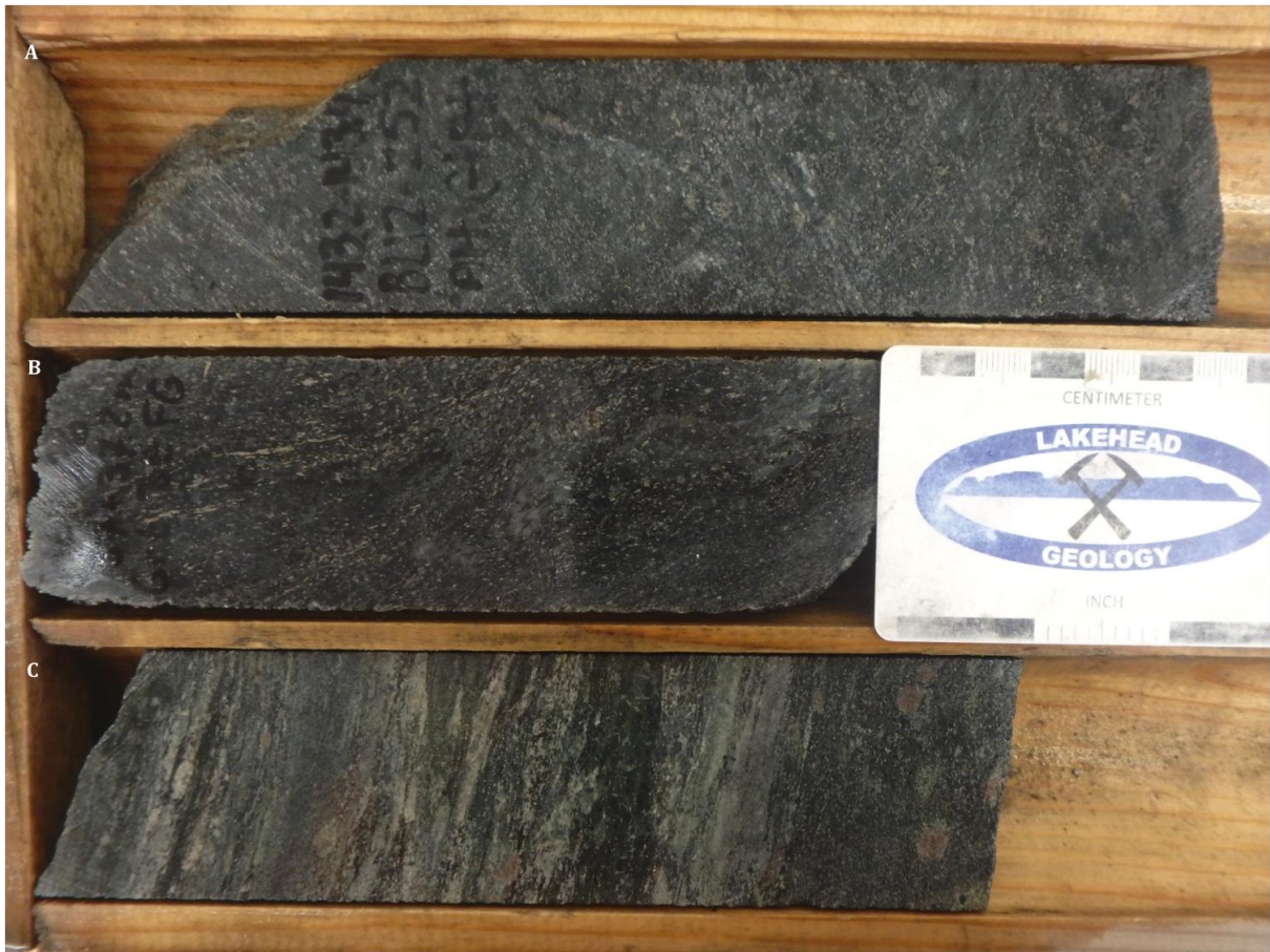
Figure 4.11. A) Fine- to medium-grained garnet-biotite schist with moderate foliation. B) Fine- to medium-grained biotite schist with a moderate to strong fabric defined by biotite and sulphide (pyrite and pyrrhotite) stringers. C) Strongly foliated garnet-biotite schist with biotite-rich melanosomes, quartzofeldspathic leucosomes and coarse garnet porphyroclasts.
