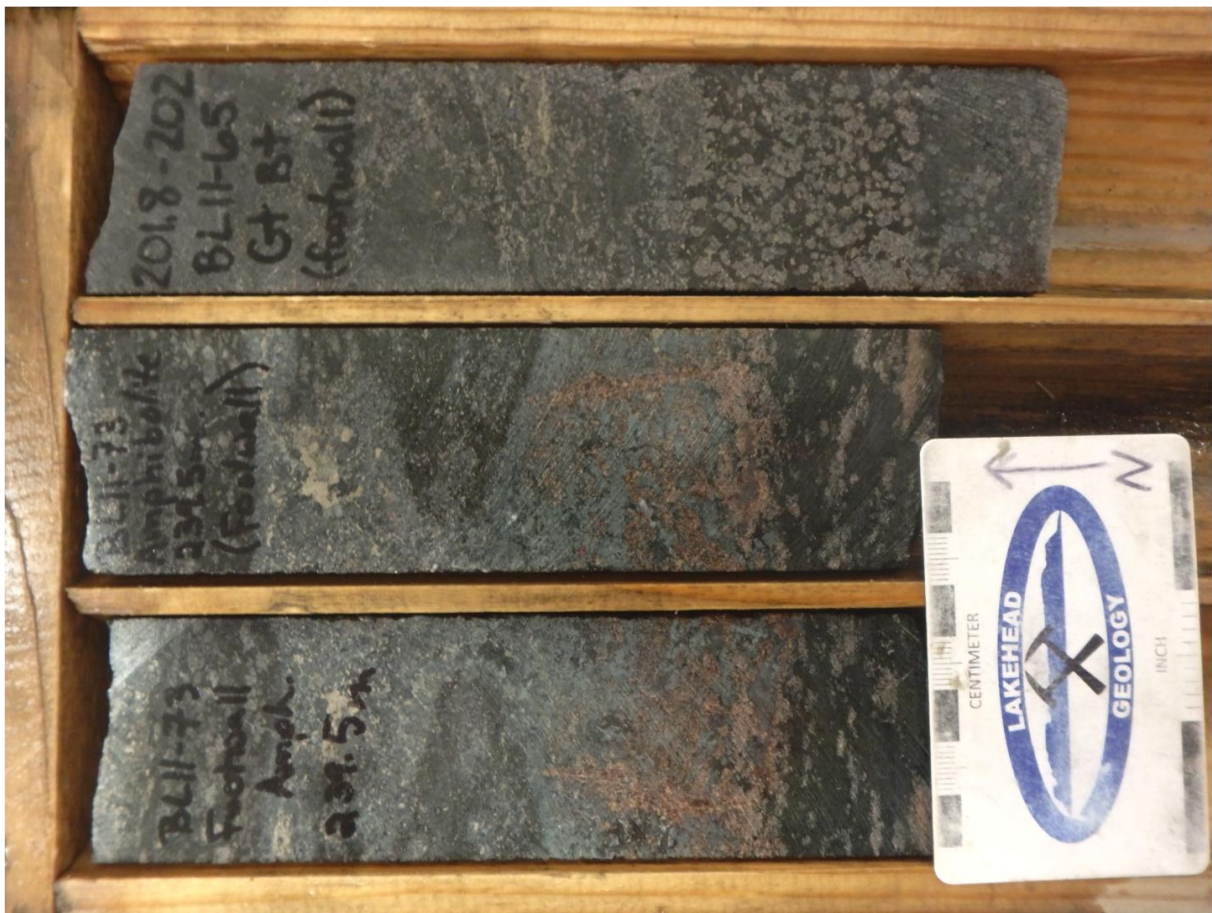
Figure 4.21. Variations in “footwall” amphibolite, consistently barren and composed of clinopyroxene, orthopyroxene, garnet and plagioclase.
