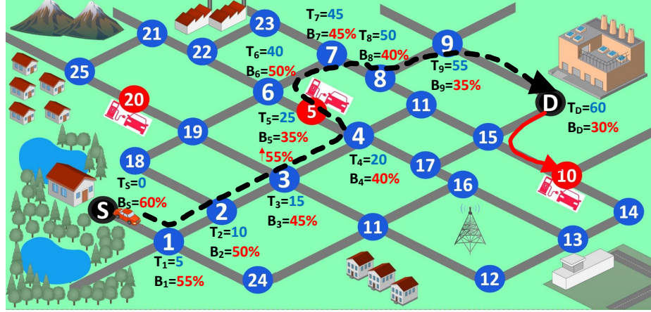
Figure 3.1: Illustration of the system model; the intersections are shown with blue nodes, charging stations with red nodes, the source and destination nodes respectively with black S and D nodes, and roads connecting nodes with links. The dotted black arrow shows the EV traveling direction on the road with arriving time ( T_i ) and battery level percentage ( B_i ) at each node.
