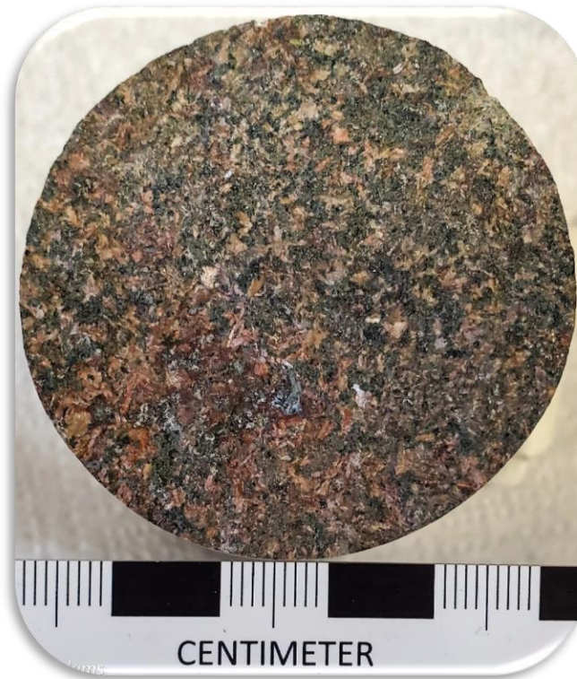
Fig 4.32: A photo of the dated monzogabbro drill core sample from the Greenwich (drill core: GL10-08).
