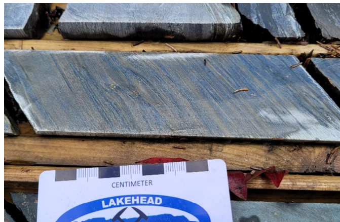
Fig 4.23 Photo of sample DT078, showing the schistose nature of the rock consisting of interbedded biotite and muscovite rich lamellae.
