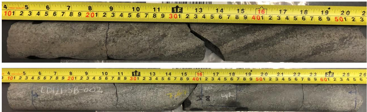
Figure 4.2. Layered, medium-grained mafic intrusive rock showing magnetite layers. Drill hole 14-902.
