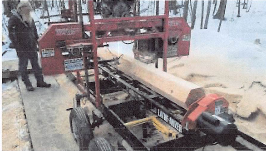
Figure 8: 6 Sided Post Created by Lathe-Mizer Attachment (Youtube)
