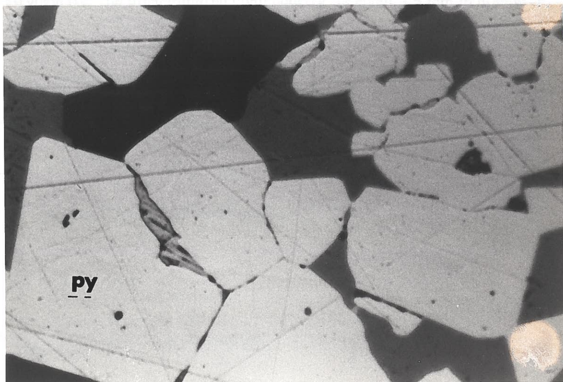
0.4mm Fig. 3.4 Annealing texture characterized by triple junctions due to recrystallization of pyrite during the slow cooling process of the deposit. Sample 49-358
