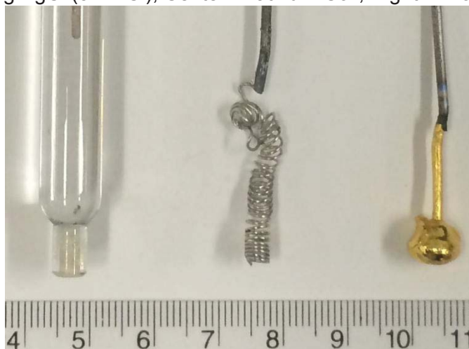
Figure 30. Electrodes assembled into 'in-house built' electrochemical cell used in capacitance experiments. Left: Ag/AgCl (3M KCl); Center: Platinum Coil; Right: Amorphous Au electrode
