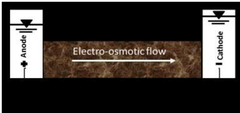
Figure 10 – Schematic of electro-osmosis in soil after (Acar, et al., 1993)
