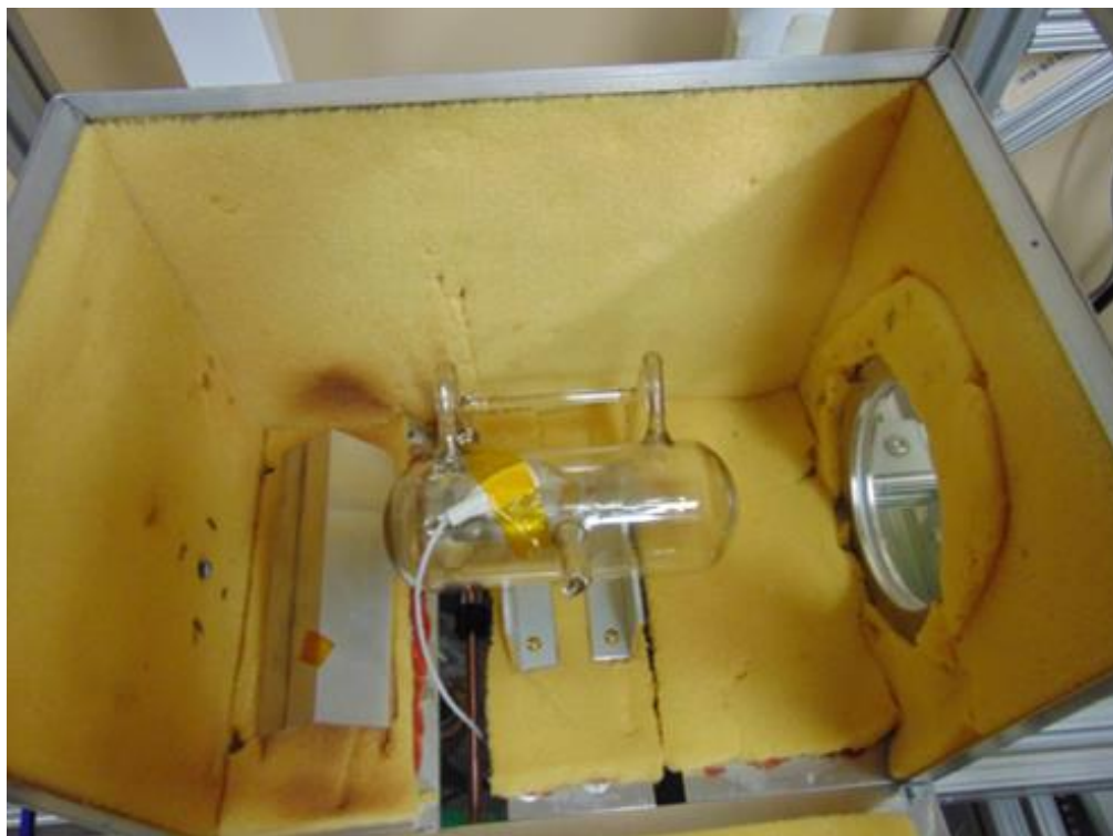
Figure 2.6. The SEOP cell inside the oven seen in figure 3.3. The entrance and the exit gates are seen on the top of the cell (with a stabilizing rod between them). The white wire connects temperature sensor. The heat supply emerges from below. The gray hue inside the cell is the rubidium.
