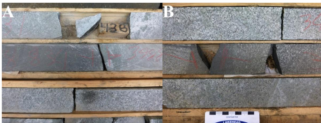
Figure 5.14. Photos of drill core from hole NOT09-2G21 displaying the variable contact relationships with their overlying and underlying ferrogabbro (down hole direction is bottom right). A. Massive oxide with sharp lower contact down hole (439 meters). B. Semi-massive oxide with sharp lower contact up hole (493 meters).
